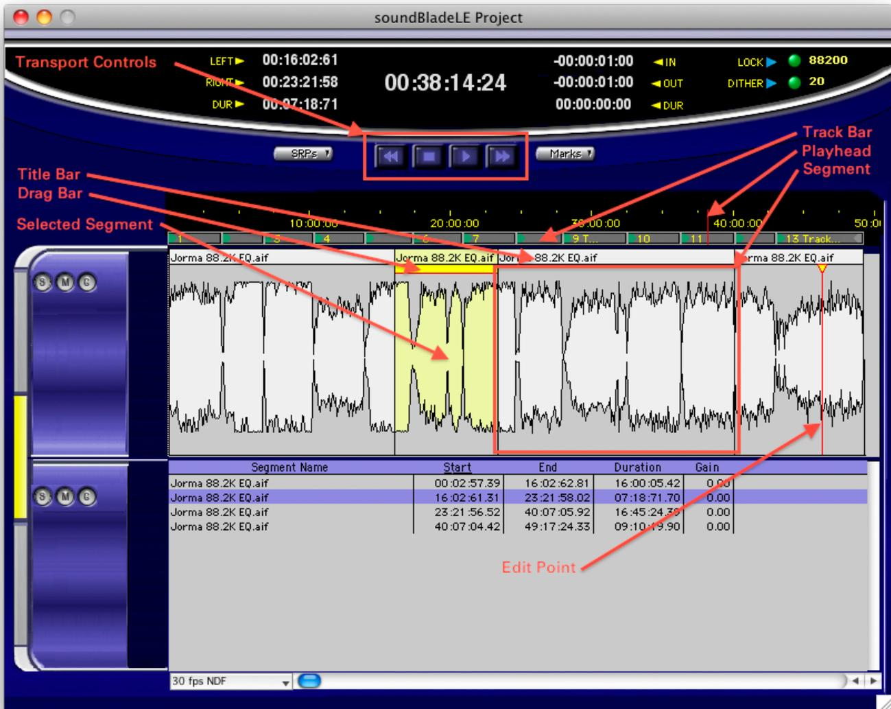
Figure 3.1: Main components of a Project window
